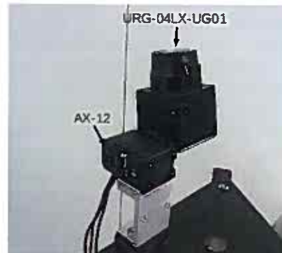
Figure 2. The tilting LRF developed
