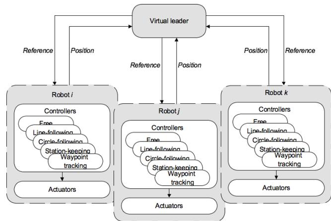
Fig. 1. An example of the developed framework with three robots
