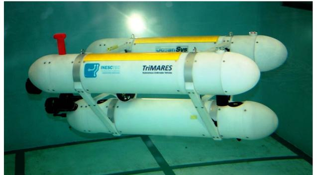
Fig. 1. The TriMARES hybrid AUV/ROV during water trials.
