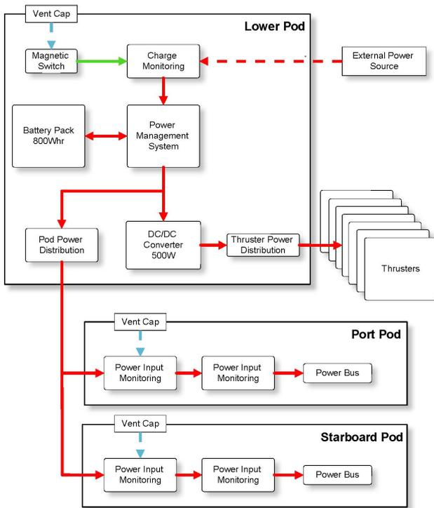
Fig. 3. Power distribution in TriMARES cylinders.
