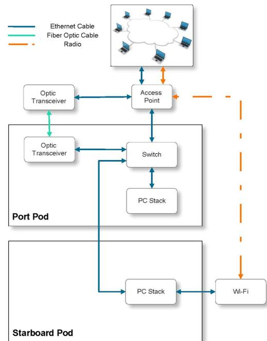
Fig. 4. Network connections in TriMARES cylinders.
