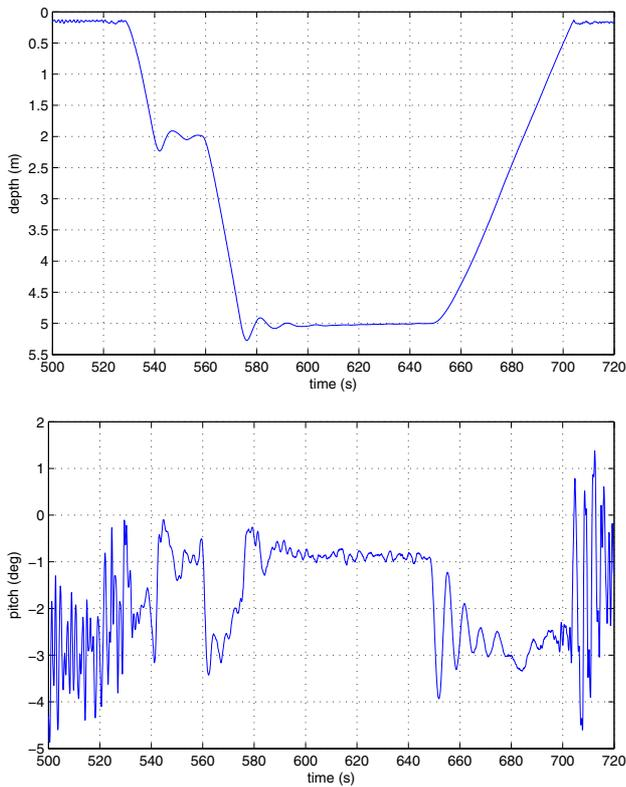
Fig. 6. Depth and pitch control of TriMARES.
