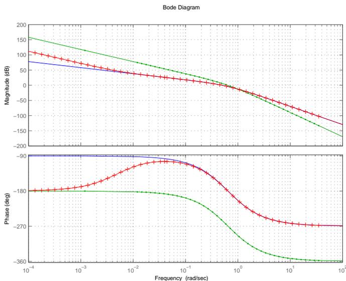
Fig. 5. Bode plots for the plant  $\frac{0.34}{s(s+0.7)(s+0.6)}$ . In solid blue, before adding any controller; in dotted-green, showing the influence of adding an extra pole at the origin; in red with the (+) signs, showing the influence of adding a pole at the origin and a zero,  $z_c = 0.005$  rad/s.
