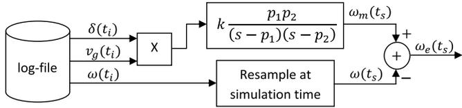
Fig. 2. Parameter identification method. The logged values of rudder angle and velocity are the input of the model. The values of angular velocity obtained using the model,  $\omega_m(t_s)$ , are compared to the values logged by the vehicle,  $\omega(t_s)$ , in order to estimate the model errors,  $\omega_e(t_s)$ .
