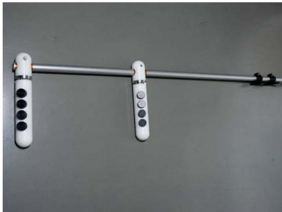
Fig. 5. Transducer array and support system.
