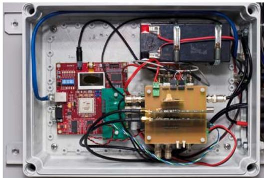
Fig. 6. Sonar signal generation and acquisition system.
