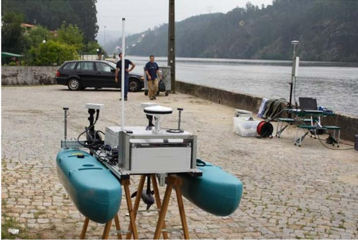
Fig. 3. Autonomous boat and base station before a mission.
