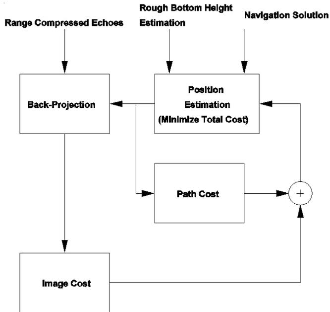
Fig. 18. Auto-focus block diagram.
