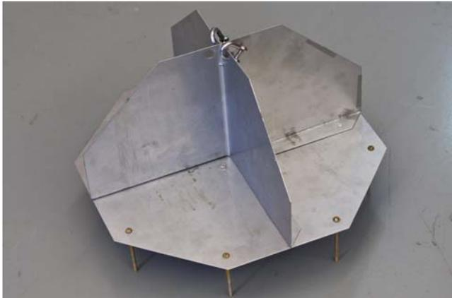
Fig. 19. Artificial target used for resolution tests.
