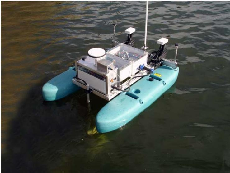
Fig. 2. Autonomous boat based synthetic aperture sonar.
