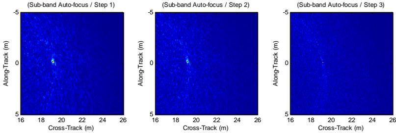
Fig. 17. Sonar image of the artificial target through the various auto-focus steps.
