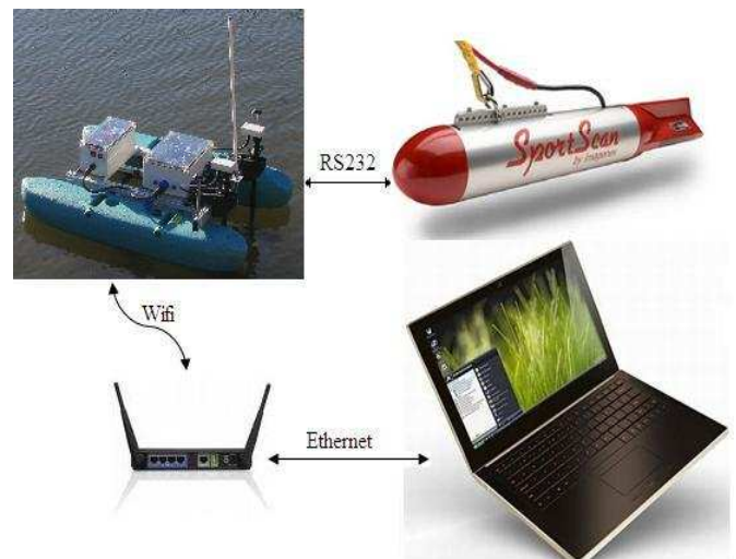
Figure 7 Communication between ImagenexSportscan, Zarco and a static laptop when the marine environment observations can be seen.
