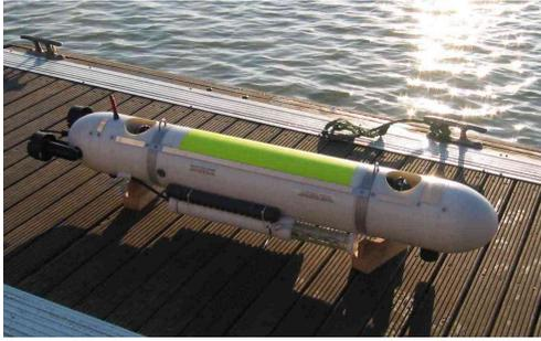
Fig. 1 MARES Autonomous Underwater Vehicle.
