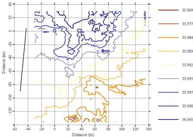
Fig. 7 Prediction contours map of salinity distribution in the vicinity of Foz do Arelho sea outfall discharge.
