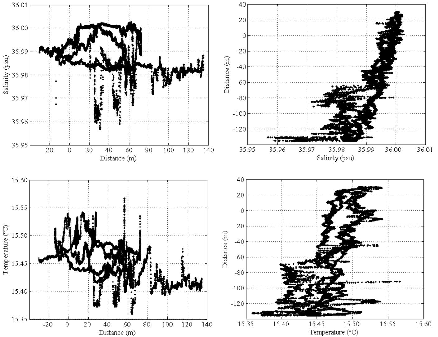
Fig. 3 Raw data of salinity and temperature measured by the AUV at 1.5 m depth.
