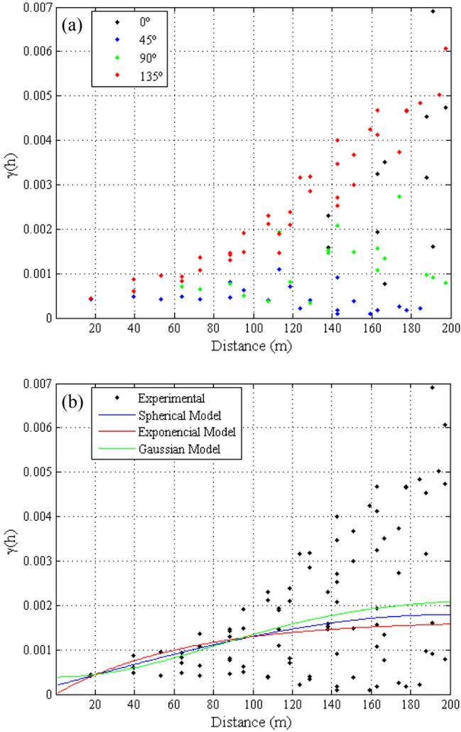
Fig. 6 (a) Directional experimental semivariogram of temperature; (b) Omnidirectional experimental semivariogram of temperature and fitted models.
