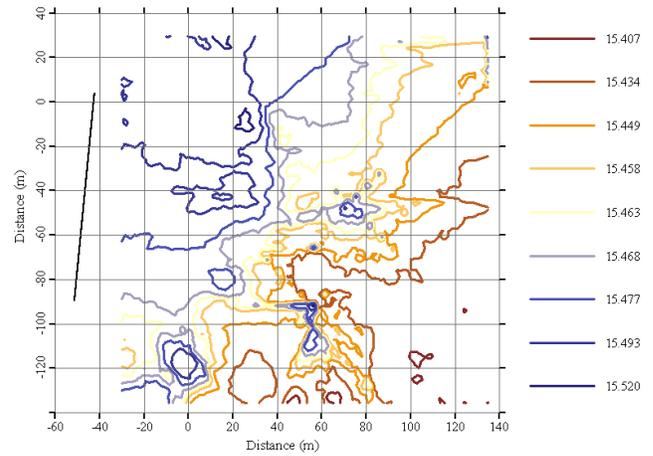
Fig. 8 Prediction contours map of temperature distribution in the vicinity of Foz do Arelho sea outfall discharge.
