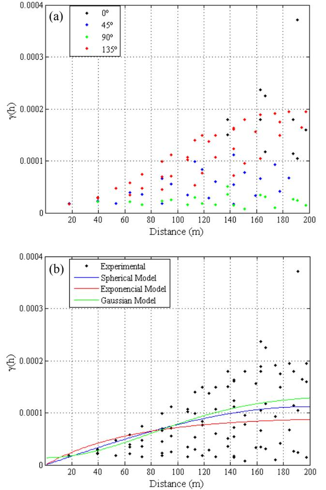
Fig. 5 (a) Directional experimental semivariogram of salinity; (b) Omnidirectional experimental semivariogram of salinity and fitted models.
