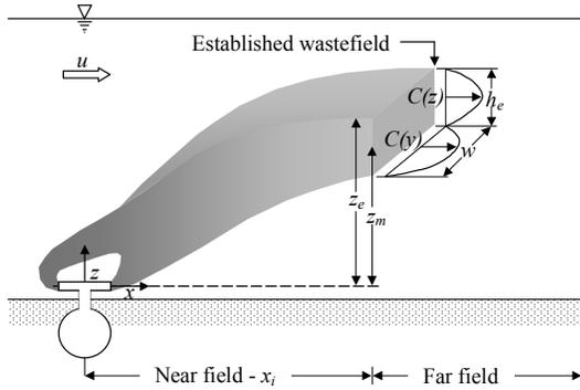
Fig. 11 Wastefield details (adapted from [2]).
