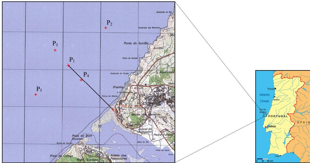
Fig. 1 Map of Foz do Arelho outfall and current measurement points.
