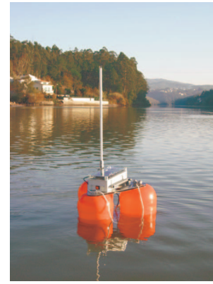
Fig. 6. Buoy connected to acoustic beacon.
