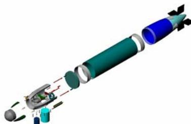
Fig. 4 - New AUV modular design
