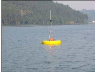
Fig. 5 - Surface buoy with underwater acoustic beacon
