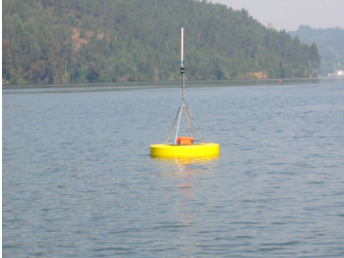
Fig. 1. Buoy with underwater acoustic beacon
