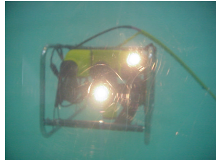
Fig. 4. Remotely Operated Vehicle for the inspection of underwater structures
